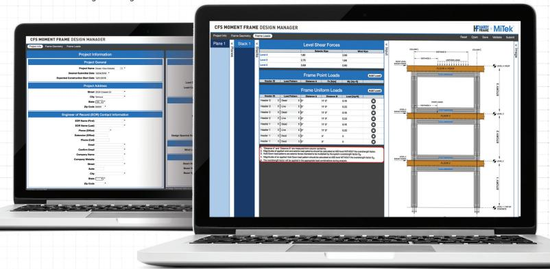
The new CFS Moment Frame Design Manager is the latest Shear Wall System software from MiTek.® It is an interactive web based program used to enter geometry and loading at vertically stacked CFS Moment Frames. User submittals go direct to our engineering department for a wall design incorporating stacked Moment Frames at multiple locations.
