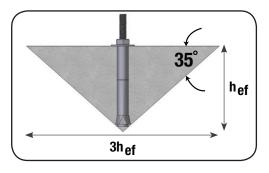
The DUC Undercut Anchor behaves nearly identically to a cast-in-place bolt. The standard embedments listed ensure that the capacity of the concrete exceeds that of the steel at the listed spacings and edge distances.
