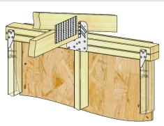
Hurricane Ties on adjacent studs to transfer roof load from top plate to wall studs. RT16 and (2) RT7A's shown.
