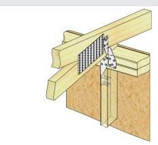
Two hurricane ties for roof to top plate and to stud to top plate connections. (2) RT7A's shown.
