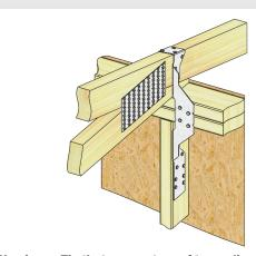
Hurricane Tie that connects roof truss directly to stud. RT20 shown.
