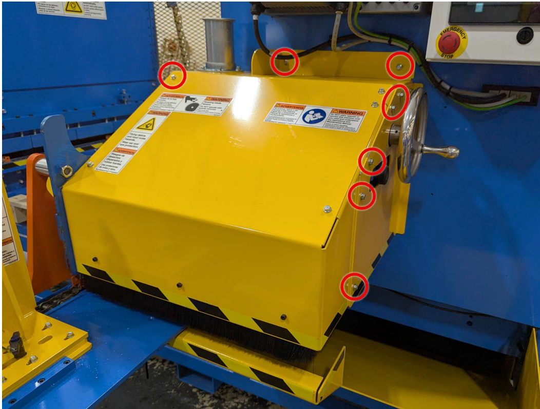
Figure 8: Bolts to Remove Cut-off Saw Housing
