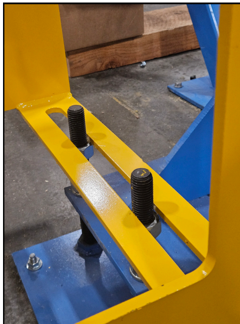
Figure 4: Platform Steps Resting on Threaded Hex Nuts
