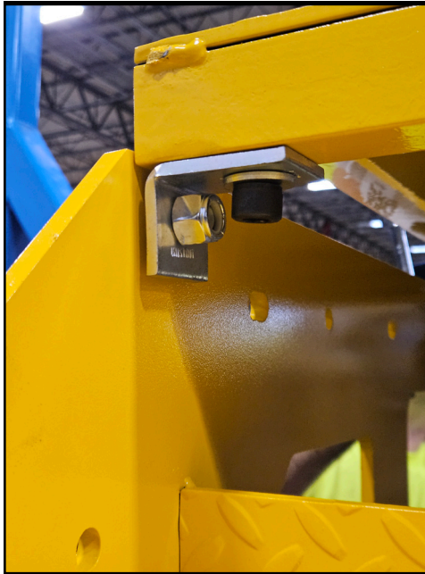
Figure 7: Telescoping Platform Secured to Steps
