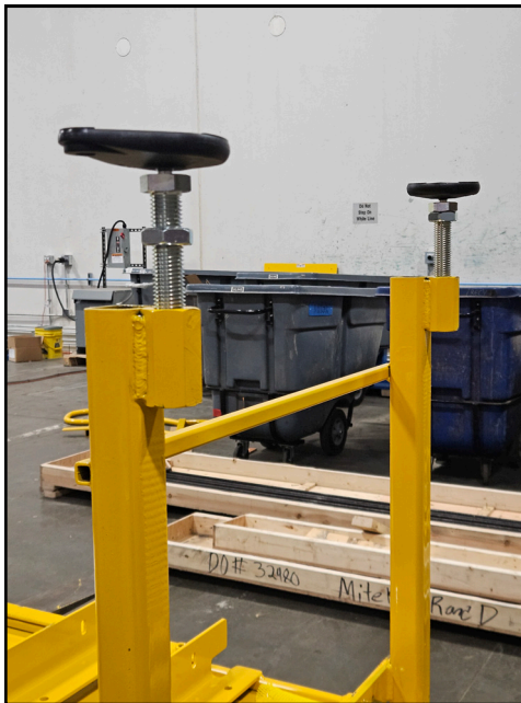
Figure 6: Leveling Feet Threaded onto Platform Stands
