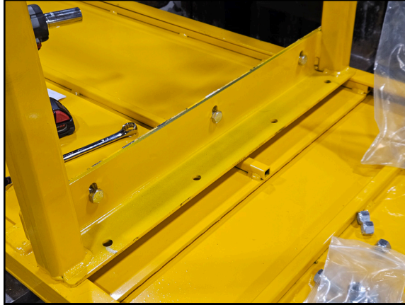
Figure 5: Platform Stands Bolted to the Stand Weldment
