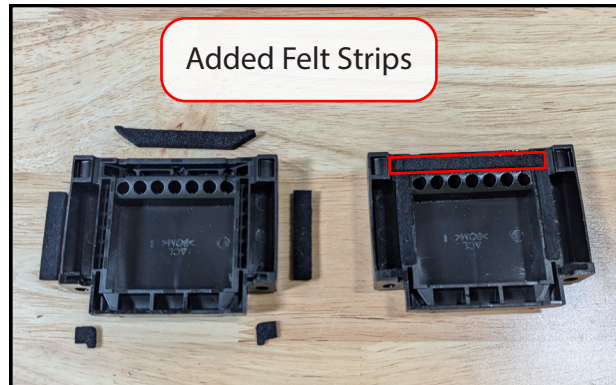
Figure 19: Dust Caps with New Felt Strips
