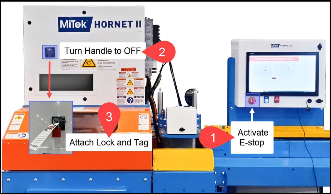
Figure 1: Hornet II Disconnect Switch Lockout/Tagout Procedure
