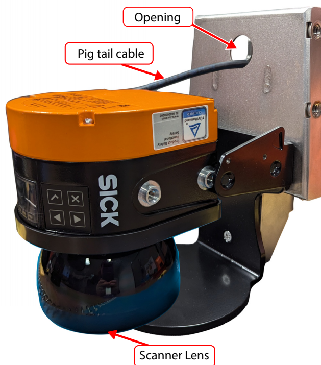
Figure 17: Slide the SICK Scanner into the Mounting Assembly
