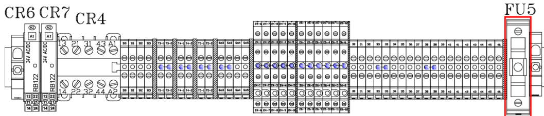
Figure 9: Fuse 5 Location Inside of Main Electrical Enclosure
