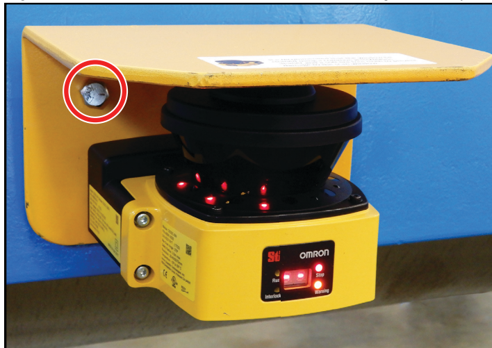
Figure 3: Bolt Locations on Omron Scanner Mounting Assembly
