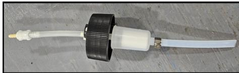
22. Run the ink line, through ink line gap in the printer, to the ink valve. Cut excess line as needed using a pair of snips.
