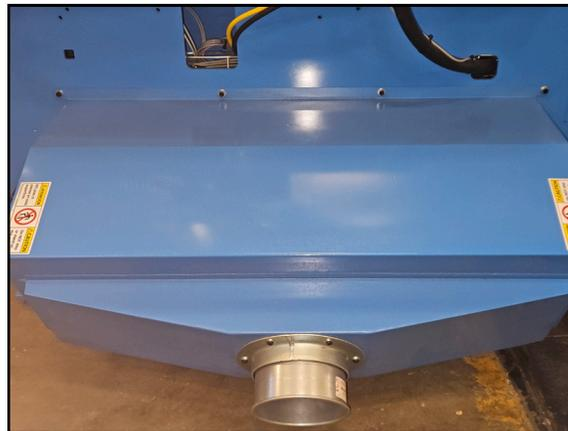
15. Where the dust hood was removed, on the right edge of the frame, feed the cables and lines into the stroke chamber through the gap in the panel.
