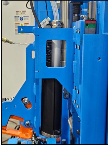
5. Attach the edge print head with the edge printer mount block.
