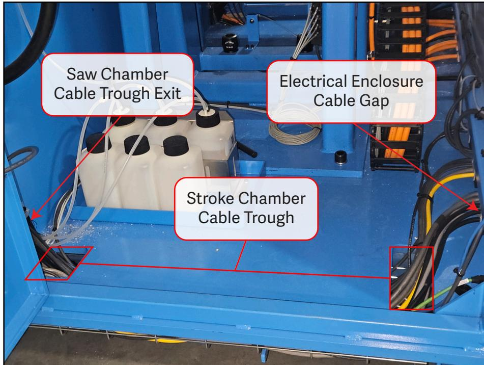
18. Feed the cable into the electrical cabinet by replacing grommets in the first gap with the supplied cable grommets ([Figure 15](#)).
