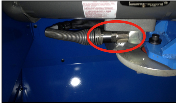
Figure 7: Connect Point at Saw Blade Motor
