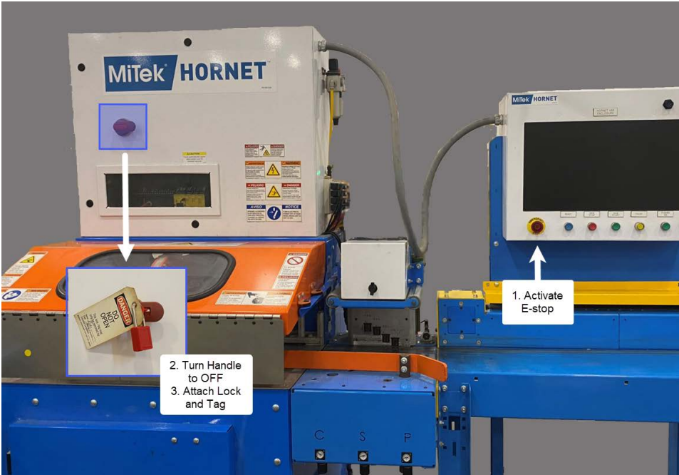
Figure 1: Hornet II Disconnect Switch Lockout/Tagout Procedure
