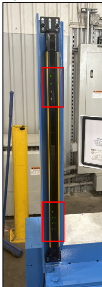
Figure 10: Receiver Indicator Lights After Successful Alignment
