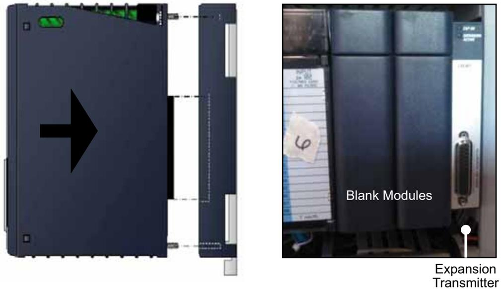
8. Install the 2 blank modules in slot #10 and #11.
