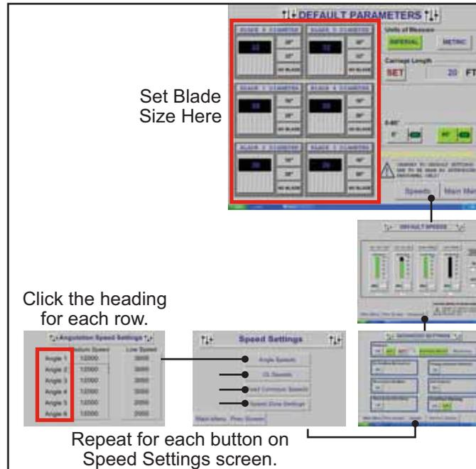
5. Calibrate the saw. Refer to the Equipment Manual for calibration instructions if necessary.
