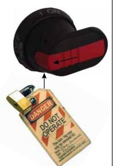
c) Lockout/tagout additional gantry heads on the same table line by repeating step 1 for each additional gantry head.
