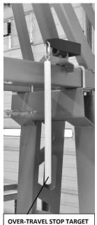
The Over-Travel Stop Targets are white plastic rods hanging from each of the end support towers. Their purpose is to interrupt the beam of one of the Obstruction Sensors and cause the trolley to stop before it hits the end bumper. They are an important part of the safety system and should not be removed.
