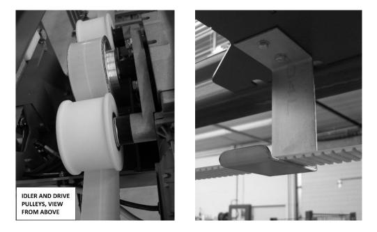
IMPORTANT: Belt must go UNDER idler pulleys and OVER drive pulley, and must lie on top of belt supports as shown.
