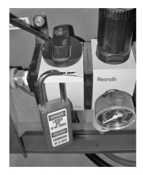
• **ELECTRICAL LOCKOUT:** To lock out the electrical system, turn the main disconnect to the off position. Push out on the hasp from behind the handle as shown, exposing padlock holes.
