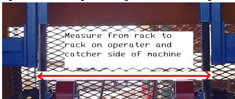
Figure B-4: Measuring the Carriage-End Hold-Down Alignment
