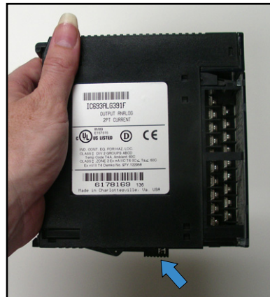
Figure 2-72: Press Release Latch to Remove Card
