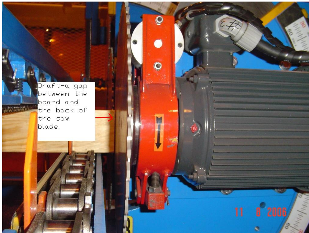
Figure B-5: The Gap Between Board and Back Half of Blade is Blade Draft
