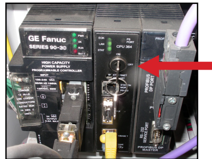
Figure 2-70: Turn Key TWICE to Reset the PLC
