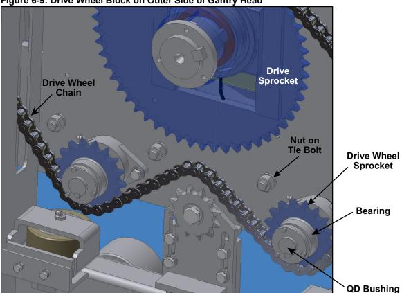
Figure 6-9: Drive Wheel Block on Outer Side of Gantry Head
