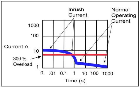
Figure F-1: Motor Inrush Curve
