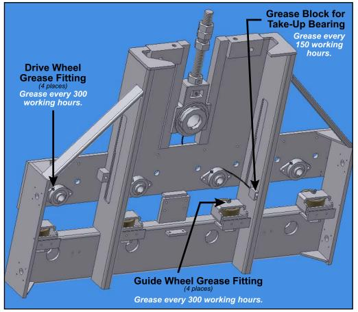
Figure 6-28: Bearing Lubrication Points, One End of Gantry Head
