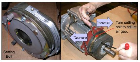
4. Check the air gap again to ensure it is now within the recommended range. It may be necessary to adjust a setting bolt more than once because the other setting bolts may affect it.
