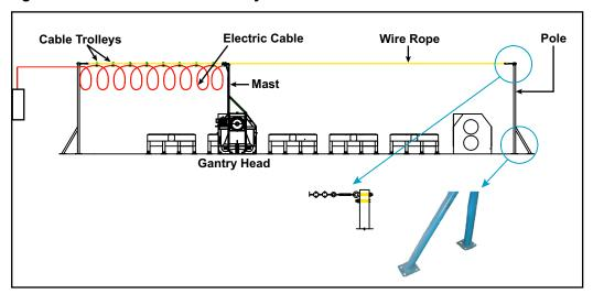
If using the pole, it is installed in the same manner that the parking stand anchor plates were installed. The pole has two (2) anchor plates, each with four (4) holes. The same anchor bolts used on the tables and conveyors will work here.
