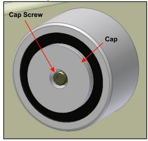
6. Replace the cap screw and tighten it to a torque of 85 ft-lbs.
