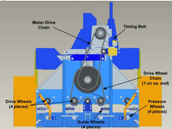
Figure 6-27: Wheels, Chains, and Belt (Machines Shipped After 15 June 2006
