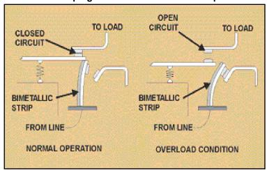
Figure F-2: The Warping Effect of the Bimetallic Strip
