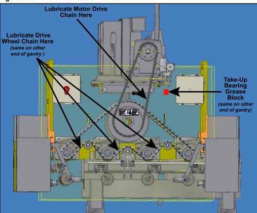
Figure 6-29: Chain Lubrication Points
