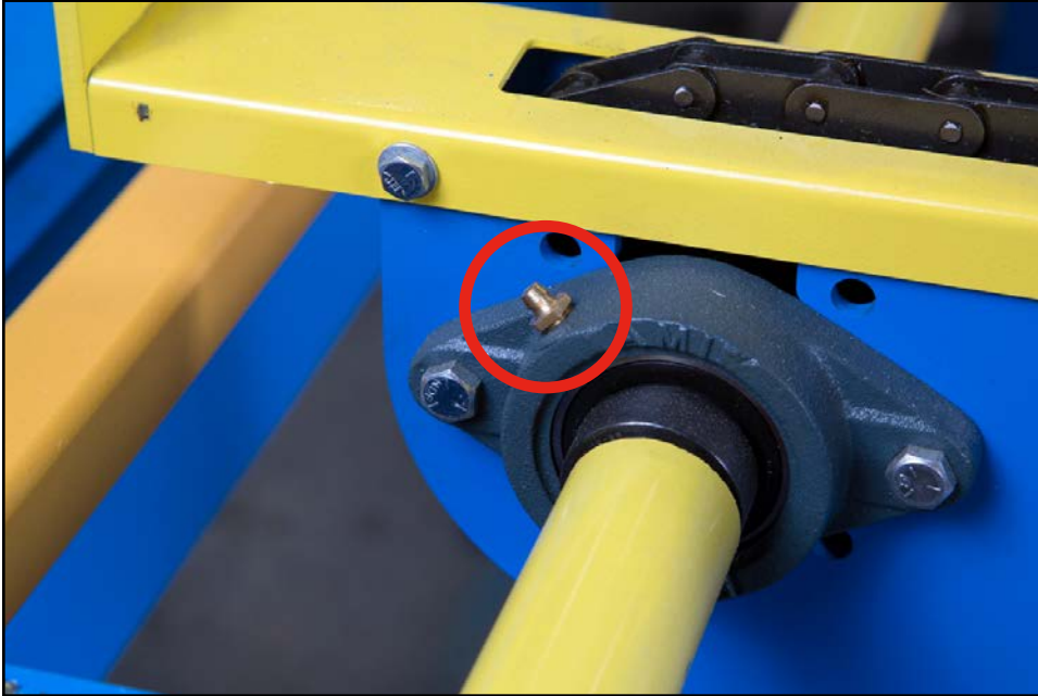
Figure 7-39: Auto Deck Drive Shaft Grease Fitting Location
