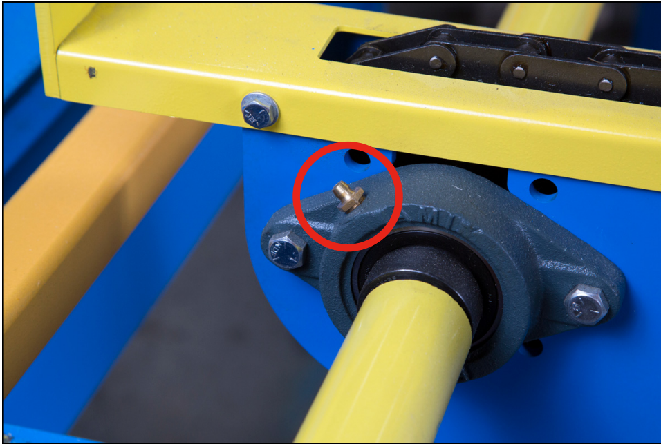
Figure 7-43: Auto Deck Drive Shaft Grease Fitting Location
