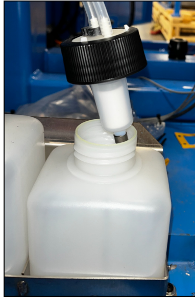
Figure 7-32: Bottle Filter and Lid Assembly
