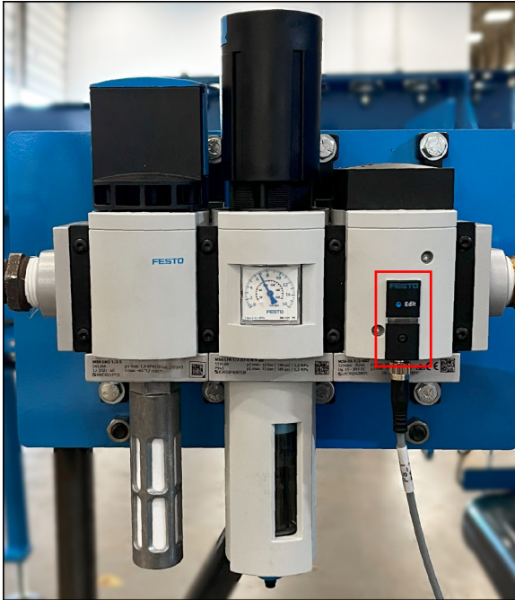
Figure 7-68: Pressure Sensor Adjustment on Main Filter/Regulator Assembly
