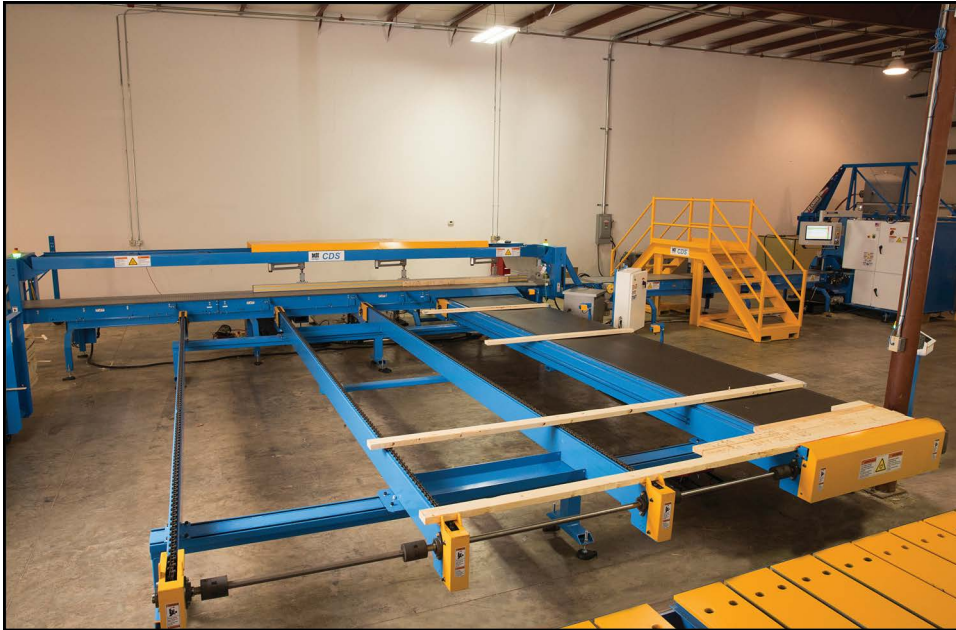
Figure 4-4: Component Delivery System (Outfeed Component)
