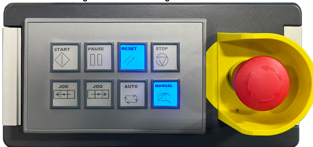
Figure 6-8: Auto Loading Live Deck Controls
