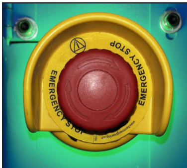
Figure 6-3: How to Operate an E-Stop Pushbutton
