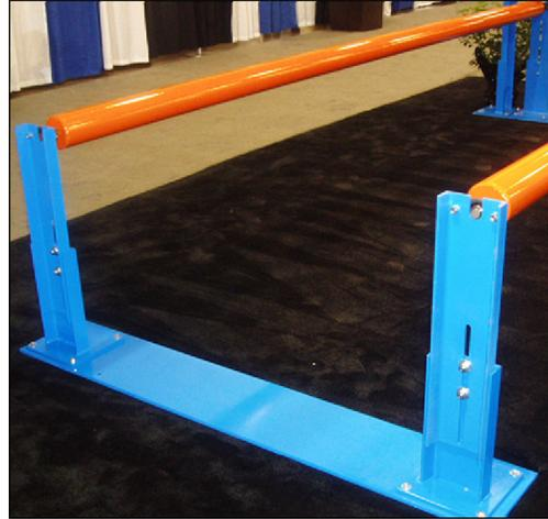
2. Set three (3) rollers, then check the diagonal dimensions to ensure they are square. See Figure 10-6. Square them with the Finish Roller before anchoring them.
