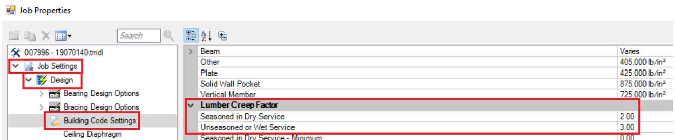
To indicate the new method of checking deflection with ANSI/TPI 1-2014 the Engineering Truss Drawing shows Vert(CT) (the Creep Total vertical deflection) instead of Vert(TL) (the Total Load vertical deflection). The horizontal deflection also changed to show Horz(CT) (the Creep Total horizontal deflection) instead of Horz(TL) (the Total Load horizontal deflection).
