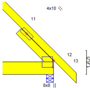
9) **WARNING:** Required bearing size at joint(s) 25, 12 greater than input bearing size.
