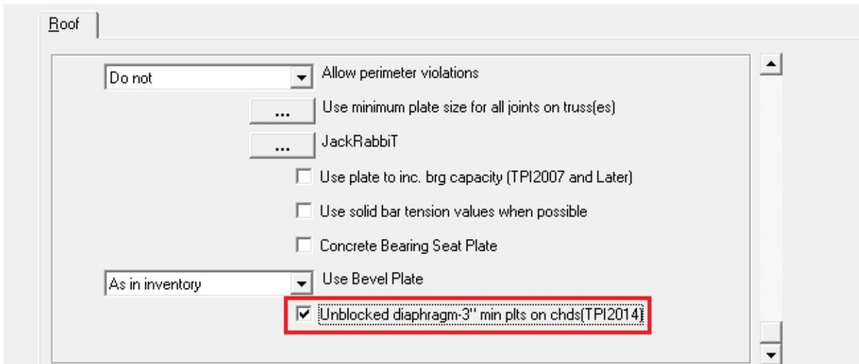
The screenshot shows the 'Roof' tab in the 'Plating Options' dialog. The 'Unblocked diaphragm-3" min plts on chds(TPI2014)' checkbox is checked and highlighted with a red box. Other options include 'Allow perimeter violations' (set to 'Do not'), 'Use minimum plate size for all joints on truss(es)', 'JackRabbit', 'Use plate to inc. brg capacity (TPI2007 and Later)', 'Use solid bar tension values when possible', 'Concrete Bearing Seat Plate', and 'Use Bevel Plate' (set to 'As in inventory').
