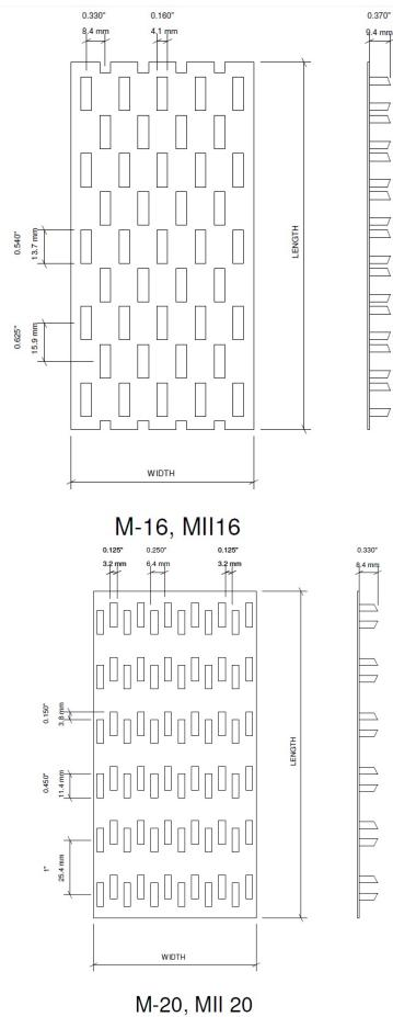
FIGURE 1—APPROXIMATE DIMENSIONS OF MITEK CONNECTOR PLATES (in inches)
