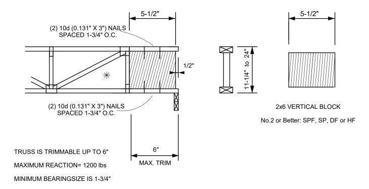
st Last diagonal web must be ran up to the top chord as shown
