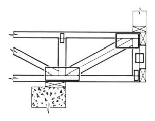
Load-Bearing Wall Cantilever Special Engineering Required
