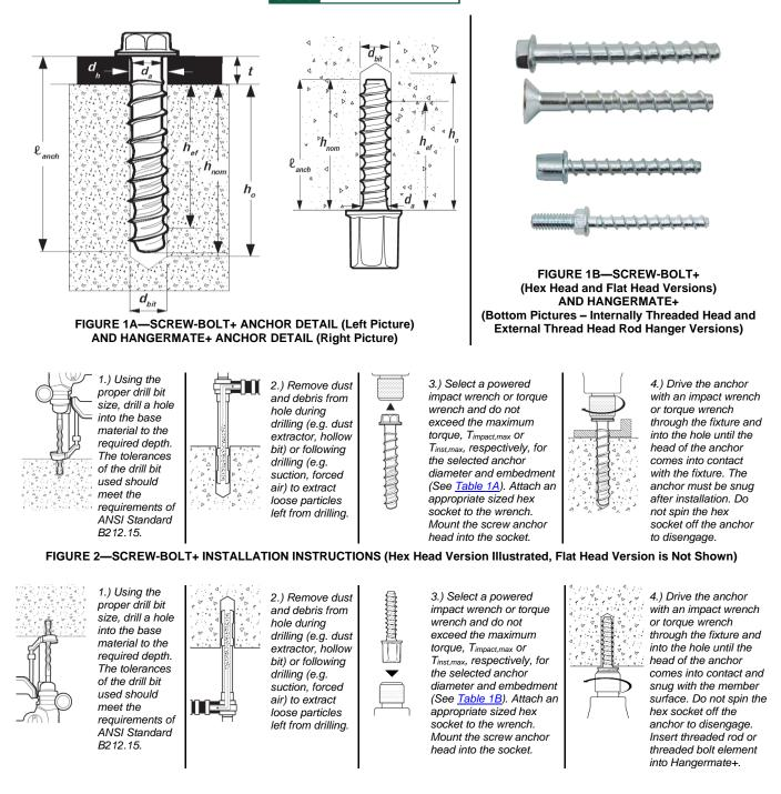
FIGURE 3—HANGERMATE+ INSTALLATION INSTRUCTIONS (Internally Threaded Rod Hanger Version Illustrated, External Thread Hanger Not Shown)
