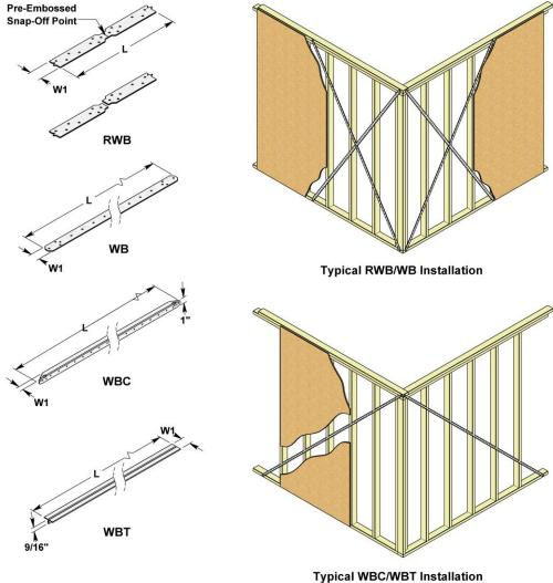
FIGURE 3-RWB, WB, WBC, AND WBT WALL BRACING
