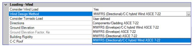
Figure 2 – Options for Wind Design Method
