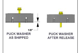
4) Before installation, the cover of the Puck Washer is raised about 1/8 inch. Compressing the washer triggers the release of the internal expansion device. In a quiet environment, you will hear an audible click when the expansion device releases.
