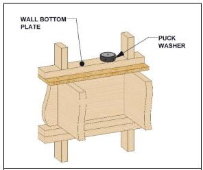
Place the Puck Washer on the wall bottom plate. The Puck Washer should be centered on the wall bottom plate.
