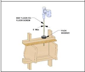
Insert the screw thru the hole in the Puck Washer and drill into the floor cavity. The screw should be driven in vertically ± 5 degrees.
