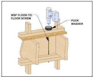
Engage the screw into the double top plate of the wall below. Tighten the screw, compressing the puck washer and releasing the internal expansion device.
