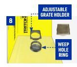
Rotate weep hole ring until flush with pan. Plastic grate holder is height adjustable to tile thickness.
