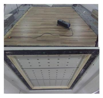
Photo 1: View of Source Chamber, finish flooring installation observed
