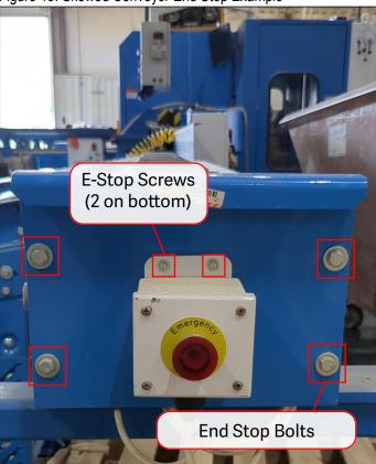
Figure 18: Skewed Conveyor End Stop Example
