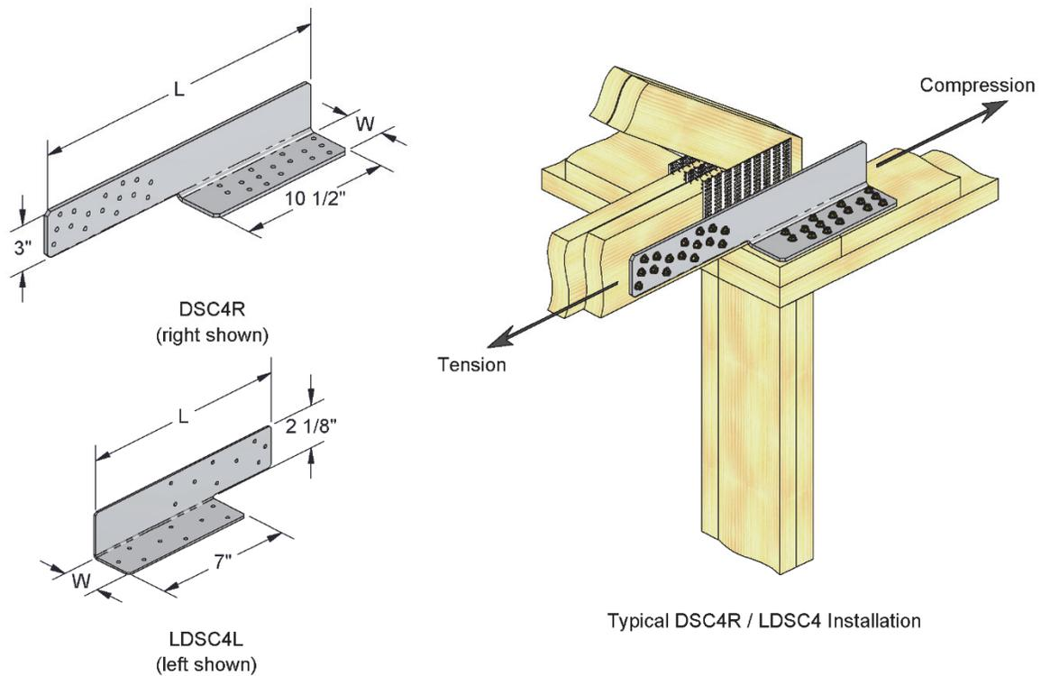
FIGURE 2—DSC AND LDSC DRAG STRUT
