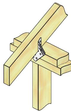
Typical RT15 truss/rafter to double plate installation
