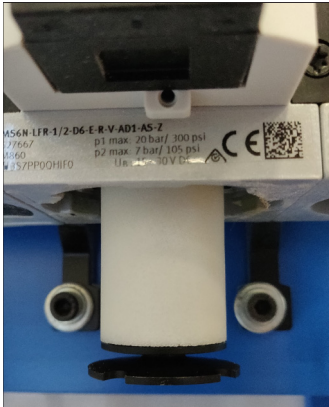
Figure 7-27: Filter Element with Bowl Removed
