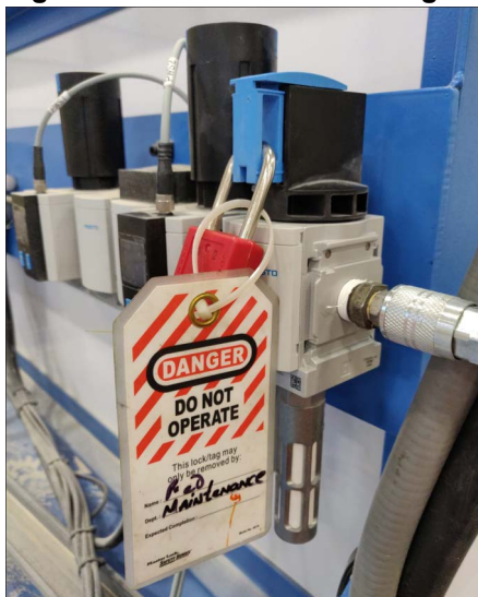
Figure 1-5: How to Lockout/Tagout the Pneumatic System
