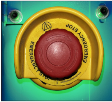
Figure 6-2: How to Operate an E-Stop Pushbutton
