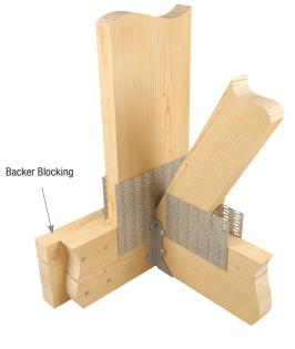
End Distance: 15 x Diameter (Dia.) Edge Distance: 2.5 x Dia. Spacing Between fasteners in a Row: 15 x Dia. Spacing Between staggered rows: 2.5 x Dia.
