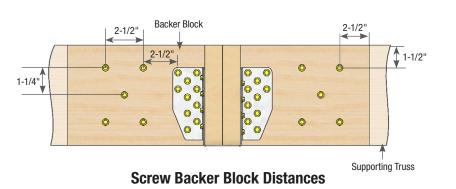
End Distance: 2-1/2" Edge Distance: 1-1/2" Spacing Between fasteners in a Row: 3" Spacing Between staggered rows: 1-1/4"
