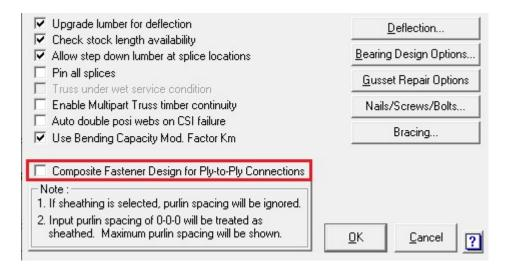
To turn off composite member design in Structure with Truss Design, in Properties dialog box select "Roof Fastener Settings", change to "Yes" in "Is Unique to Truss" in General section and to "No" in "Composite Fasteners Design for Ply-to-Ply Connections" in Connection Options section.
