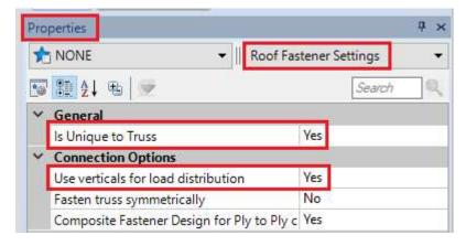
After selection is made, Redesign the truss. If you have the "Use verticals for load distribution" already on and get a ply-to-ply connection note, try to turn the "Use verticals for load distribution" off, may be vertical is too short to transfer load, and Redesign the truss.
