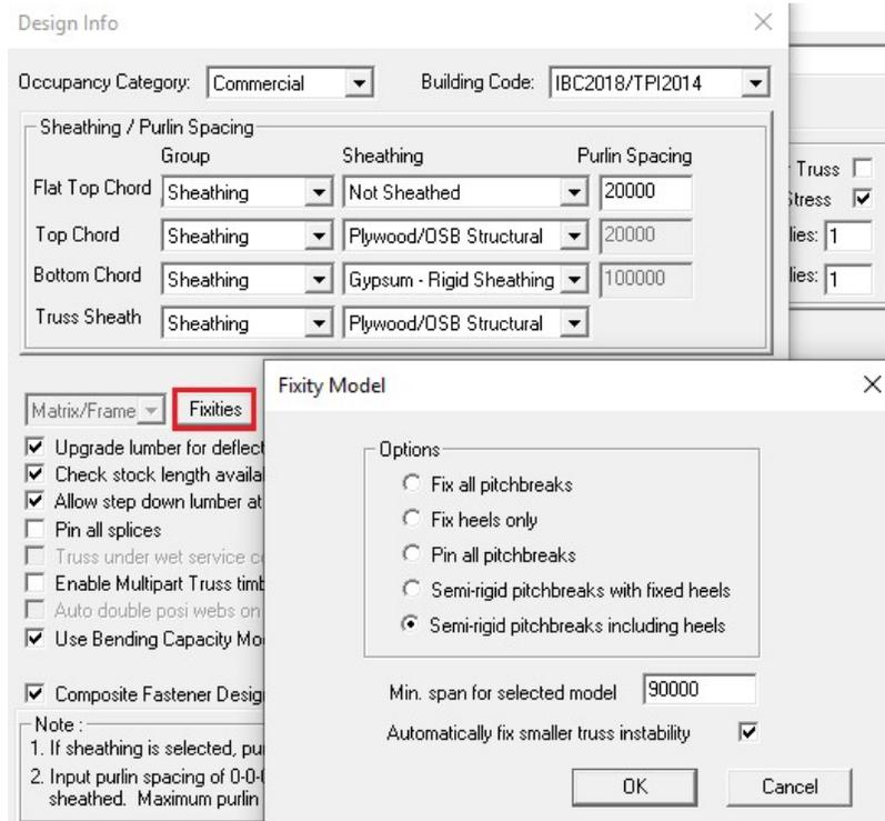
And in the File – Setup – Job Properties – Job Settings – Design – Fixities section on Job level in Structure with Truss Design:
