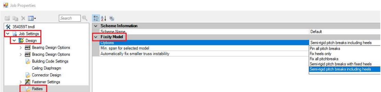
And in The Properties – Fixities section on Truss level:
