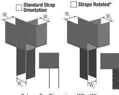
$W_1, W_3, W_4$  will typically be 1/8"–1/4" greater than beam widths.  $W_2$  will typically be 0"-1/8" greater than post width.
