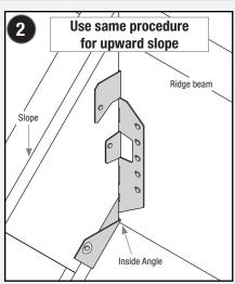
Lean hanger and rafter end against ridge beam at desired position. Install 10d (0.148" x 3") HDG or 16d (0.162" x 3-1/2") HDG nails through nail holes into ridge beam at right  $90^{\circ}$  angle. If skewing the rafter, only drive HDG nails into ridge beam on inside flange.
