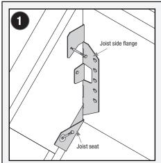
Position LSSH hanger against plumb-cut end of joist as shown. Fasten joist side flanges on both sides with 10d (0.148") x 1-1/2" HDG nails. Bend seat up to fit against joist bottom and drive (1) 10d (0.148") x 1-1/2" HDG nail through bottom seat into rafter bottom.
