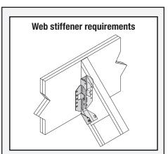
Web stiffeners are required for all wood I-Joist installations. Designer may consider adding a tension restraint for the supported member for roof slopes exceeding 6/12.
