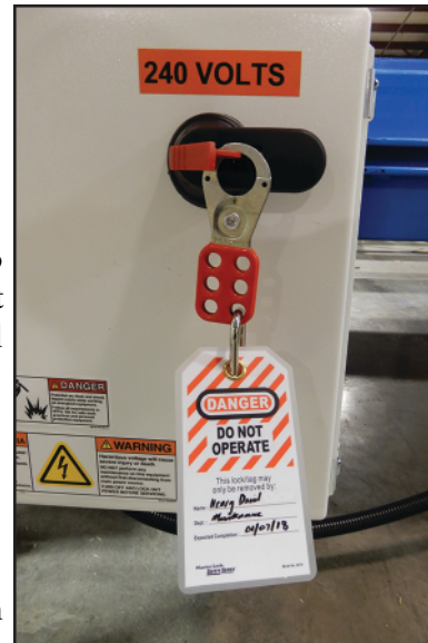
Figure 1-1: An Example of a Lockout/Tagout Device
