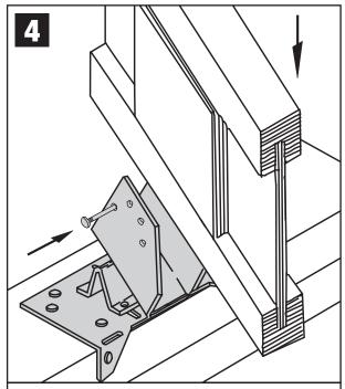
Insert rafter into Rafter Pocket. Use downward pressure to fully seat the rafter. Adjust rafter and pocket to correct pitch. Fasten rafter to rafter pocket with (8) 10d (0.148") x 1-1/2" nails.
