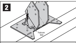
Fasten connector to the top of top plate with (6) 10d (0.148" x 3") nails. **NOTE:** Do not drive nails through fulcrum slots yet.
