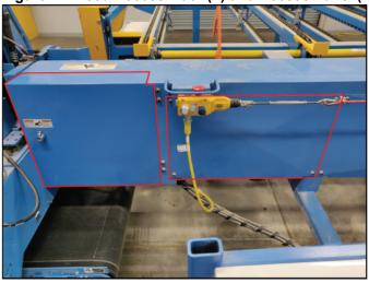
3. Remove all visible cable ties and wrap behind both panels. The cables will be connected and re-bundled at a later point.
