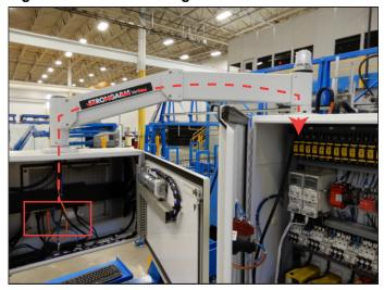
c) Locate the **50-ft Cat5/6 cable** in the bottom *BLADE* main electrical enclosure and route the free end into the top enclosure through the connecting hole. The cable will be fished through the conduit opening (circled in Figure 10).
