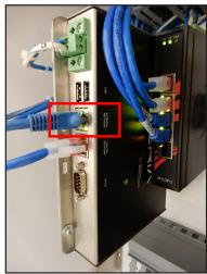
9. Connect all **print head cables** inside the *MPERIA* enclosure. The cables should be labeled with a letter (A or B) and their associated print head location (Front, Rear, or Edge). The V-Link PRINTHEAD ports are labeled A or B. See Figure 17.
