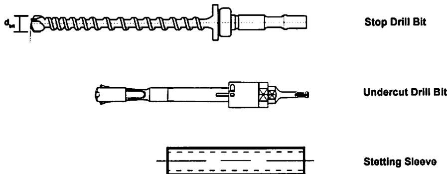
FIGURE 4—STOP DRILL BIT, UNDERCUT DRILL BIT AND SETTING SLEEVE
