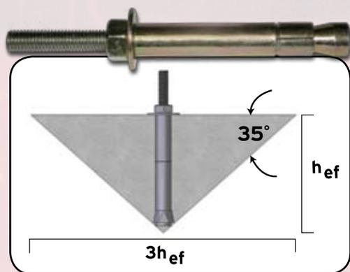
The DUC Undercut Anchor behaves nearly identically to a cast-in-place bolt. The standard embedments listed ensure that the capacity of the concrete exceeds that of the steel at the listed spacings and edge distances.
