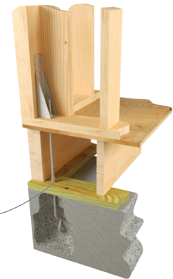
Typical CNW installation
