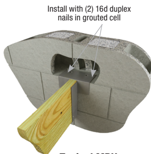
Typical MPH single-ply installation
