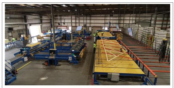
With just over one year in the field, the MatchPoint® DirectDrive™ system is reducing shop floor labor by up to 40% for its users.
