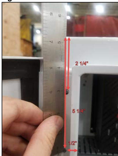
Figure 3: MPA Heater Enclosure Mounting Hole Position/Location
