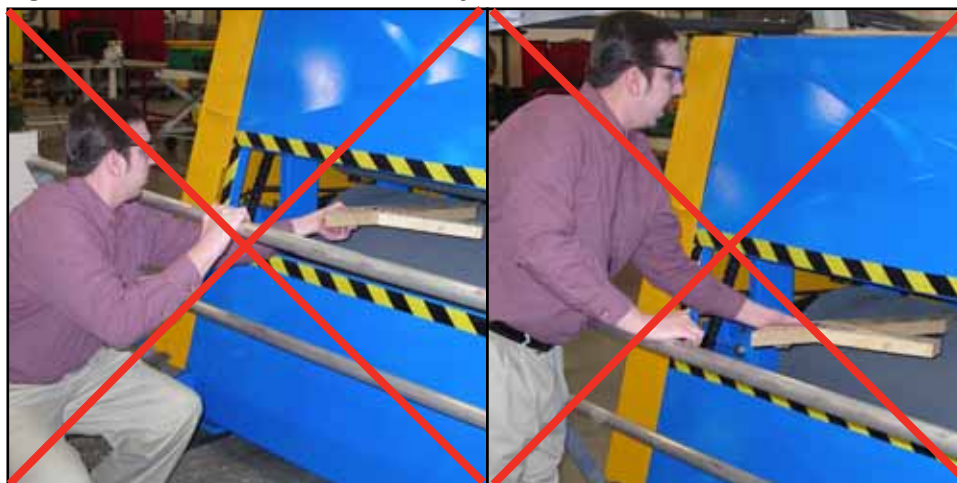
Figure 13: Do Not Hand-Feed Directly Into Finish Roller
