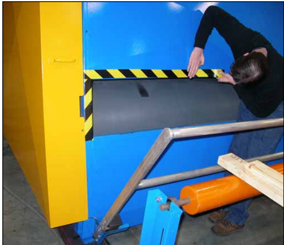
Figure 3: Applying the Warning Tape
