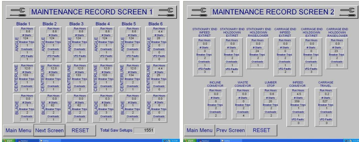
The Maintenance Record Reset screen is used to reset the data on the Maintenance Record screens 1 and 2 back to zero (0). This feature is useful during troubleshooting. The data is not archived, so ensure you will not need it before resetting data.
