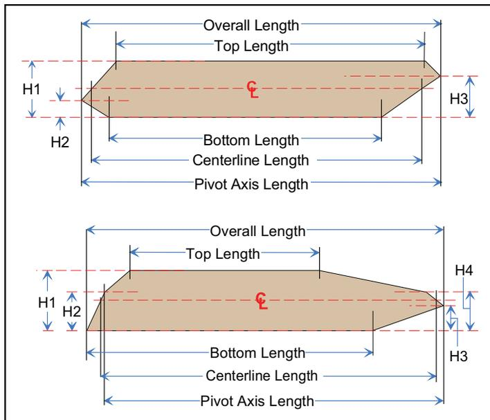
Figure 2-3: Parts of a Truss
