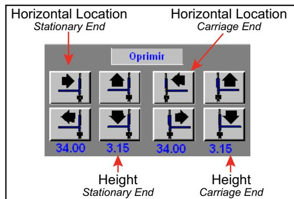
When operating in Automatic Mode, the hold-downs are automatically set to be a specific distance from the saw blades. To override this automatic setting, refer to the *Setting the Infeed Conveyor Offset* section on page OP-68.
