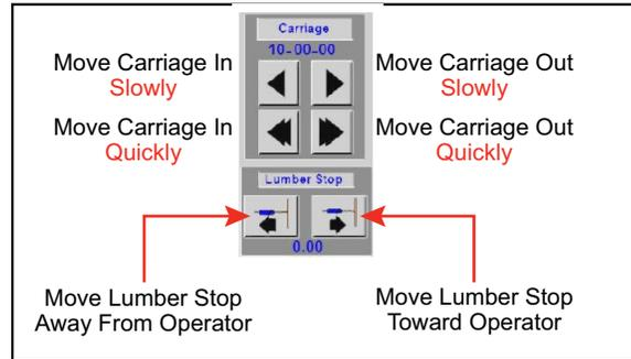
When operating in Automatic Mode, the carriage automatically moves to the correct position for the programmed cut.
