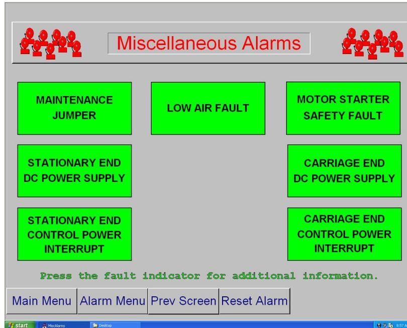
All of the miscellaneous alarms are reset automatically when the alarm condition is cleared.
