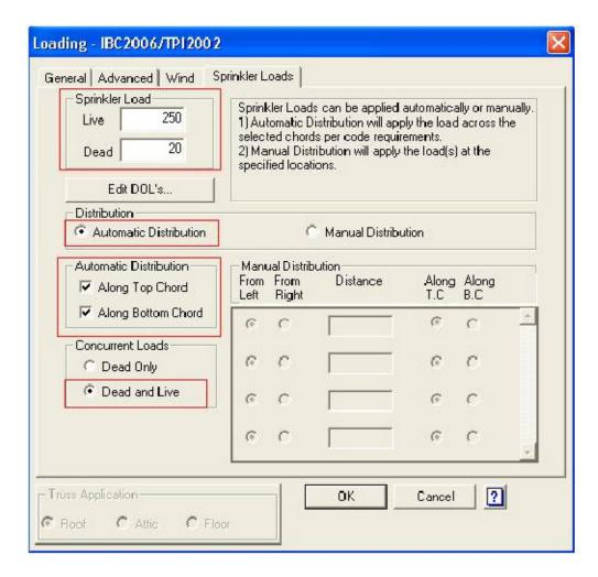
Select OK. Program will automatically apply specified load to each panel point and mid-panel point in separate load cases.
