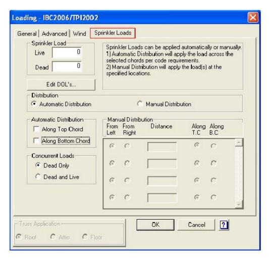
Since the truss is already designed to handle the dead loads from the Fire Sprinkler System (included in the Top Chord Dead Load), it only needs to be checked for the additional 250 pound live load (weight of sprinkler installation personnel) which is nonconcurrent with any other live loads. Specify 250 for Live and 0 for Dead. Choose Automatic Distribution. Then specify distribution of Sprinkler Load Along Top Chord and Concurent Loads as Dead Only.
