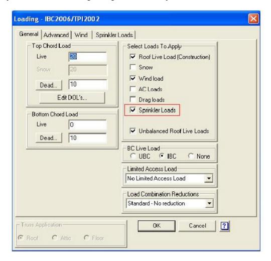
Then click on the Sprinkler Loads tab at the top of the Loading Dialog box. Specify 250 pound Live Load (weight of sprinkler installation personnel) and 20 pound Dead Load (weight of water-filled pipe). Choose Automatic Distribution. Then specify distribution of Sprinkler Load Along Top Chord and Along Bottom Chord and Concurent Loads set to Dead and Live.
