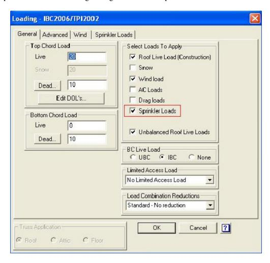
Then click on the Sprinkler Loads tab at the top of the Loading Dialog box. Specify 250 pound Live Load (weight of sprinkler installation personnel) and 50 pound Dead Load (weight of water-filled pipe). Choose Manual Distribution and then specify location of concentrated load at 6' From Left Along Top Chord and Concurrent Loads set to Dead and Live.
