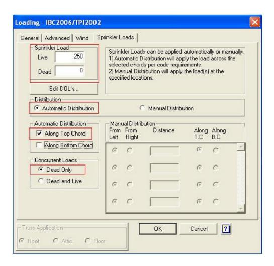
Select OK. Program will automatically apply specified load to each panel point and mid-panel point in separate load cases. This is a conservative approach, but it ensures that this live load has been covered for any variance in the installed location of the sprinkler system hangers.
