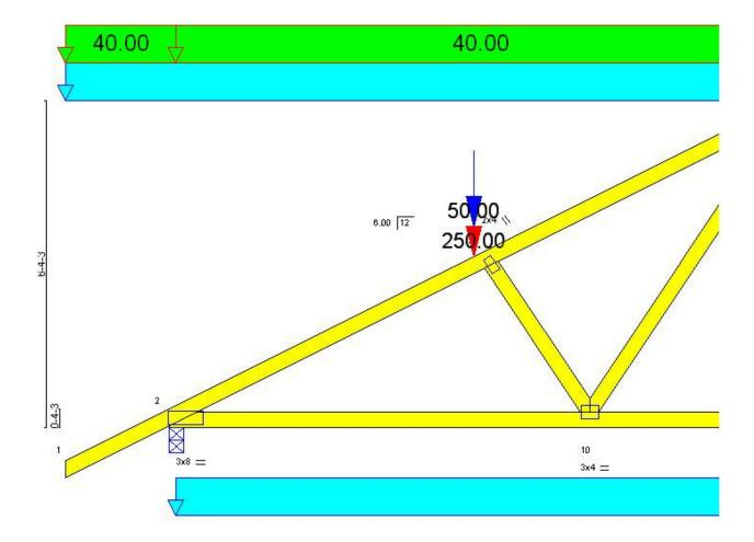
There should be no more than one Fire Sprinkler System support attached to each truss panel. If more than one Fire Sprinkler System support is needed in one panel or loading for Fire Sprinkler System indicated on the plan is not covered in this article please contact Engineering Office.
